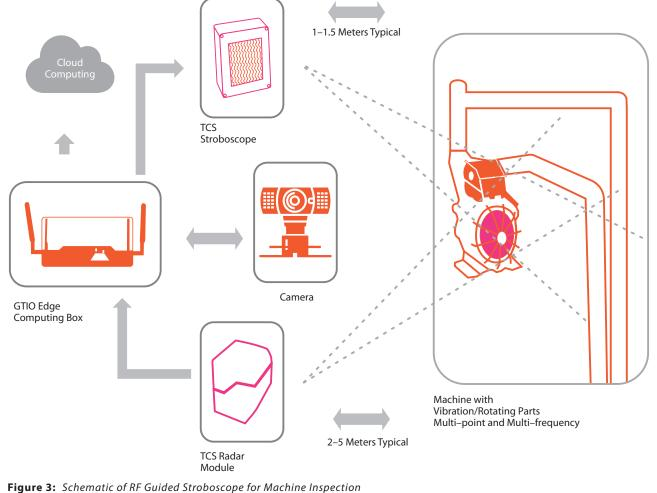
Figure 5. Schematic of KF Galded Stroboscope for Machine Hispect
